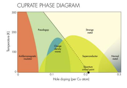
Figure 1: The phase diagram of typical high  $T_c$  superconductor
