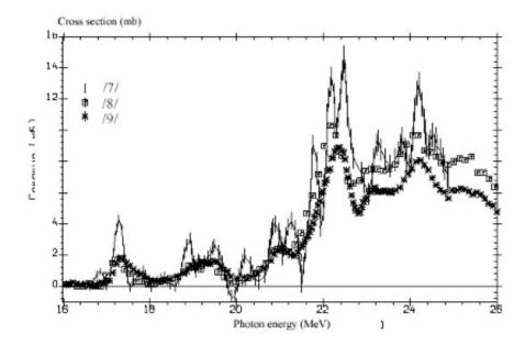
**Figure 1:** The comparison of photoneutron cross sections  $^{16}O(\gamma, xn)$  obtained in one BR-experiment (Moscow State University) and two QMA experiments carried out at Saclay (France) Livermoore (USA). Figure is taken from [C4] where also references to experiments can be found.
